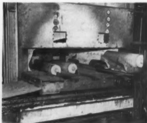
Dogs push shells into a Gas Machinery Co. retarded-cooling furnace. Shells mount on mandrels, are righted and go through vertically. Heating elements along furnace walls prevent excessive cooling of outside shells, cool them at the same rate as those in the center rows
